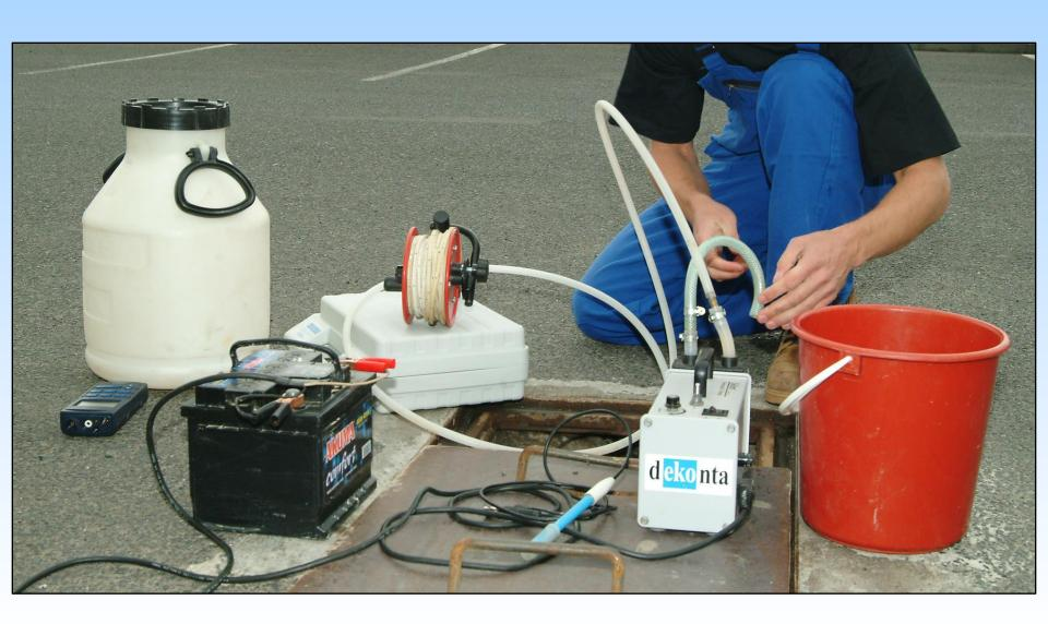
From the sampled well is pumped required amount of water, usually 3-5 volumes before sampling.
