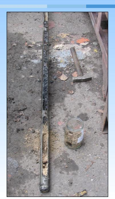
Soil sample taken from the core of the sampler
