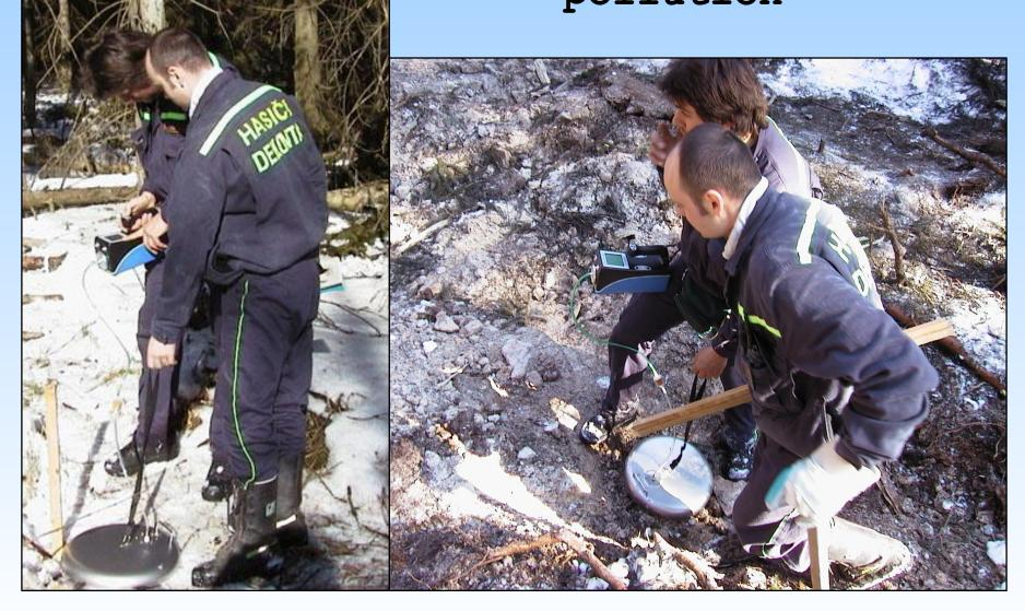
Pollutant concentration measuring - ECOPROBE venting well; air flow measurement - rotameter
