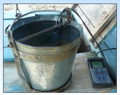
The described procedure is applicable for sampling from unequipped wells and in justified cases also from equipped wells. The use of static way is given by specific conditions, eg:
